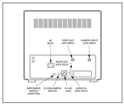
Figure 1. Rear Panel Connections
